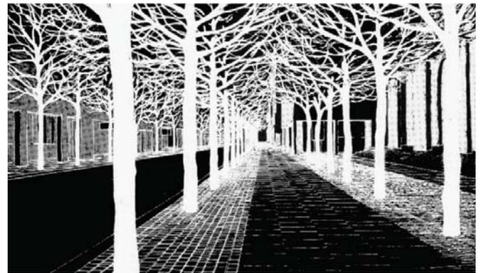
*Correct tree form and placement provides side as well as overhead enclosure.*
