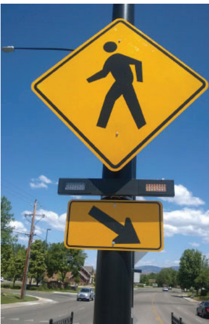
rectangular rapid flashing beacon
